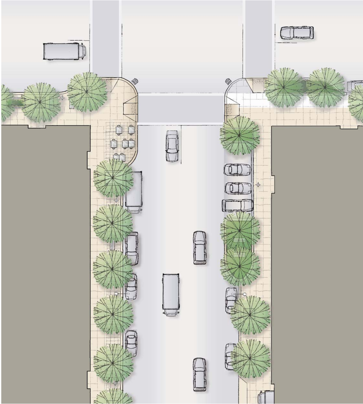
Figure E.3. Mixed Use street showing stormwater planters, perpendicular parking, and seating areas
