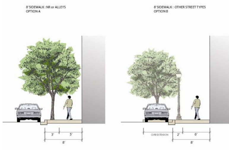
Caption: Two options for dividing an 8' wide sidewalk: a) On alleys or neighborhood residential streets, retain a minimum 4' through-way, and plant trees in the furnishings zone (min. 3'); b) On other street types, retain a 6' through-way, use narrow elements such as streetlights or bollards in the furnishing zone, and add optional curb extensions with street trees.
