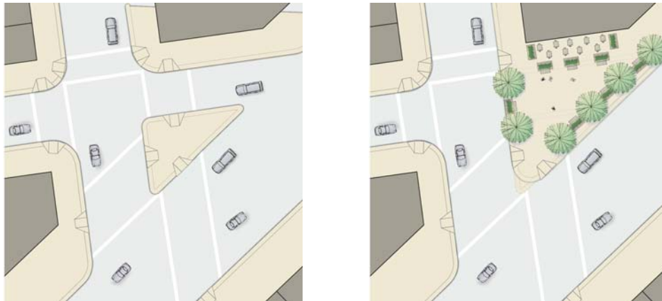
Figure F.2. Conversion of a corner slip lane into a public space
