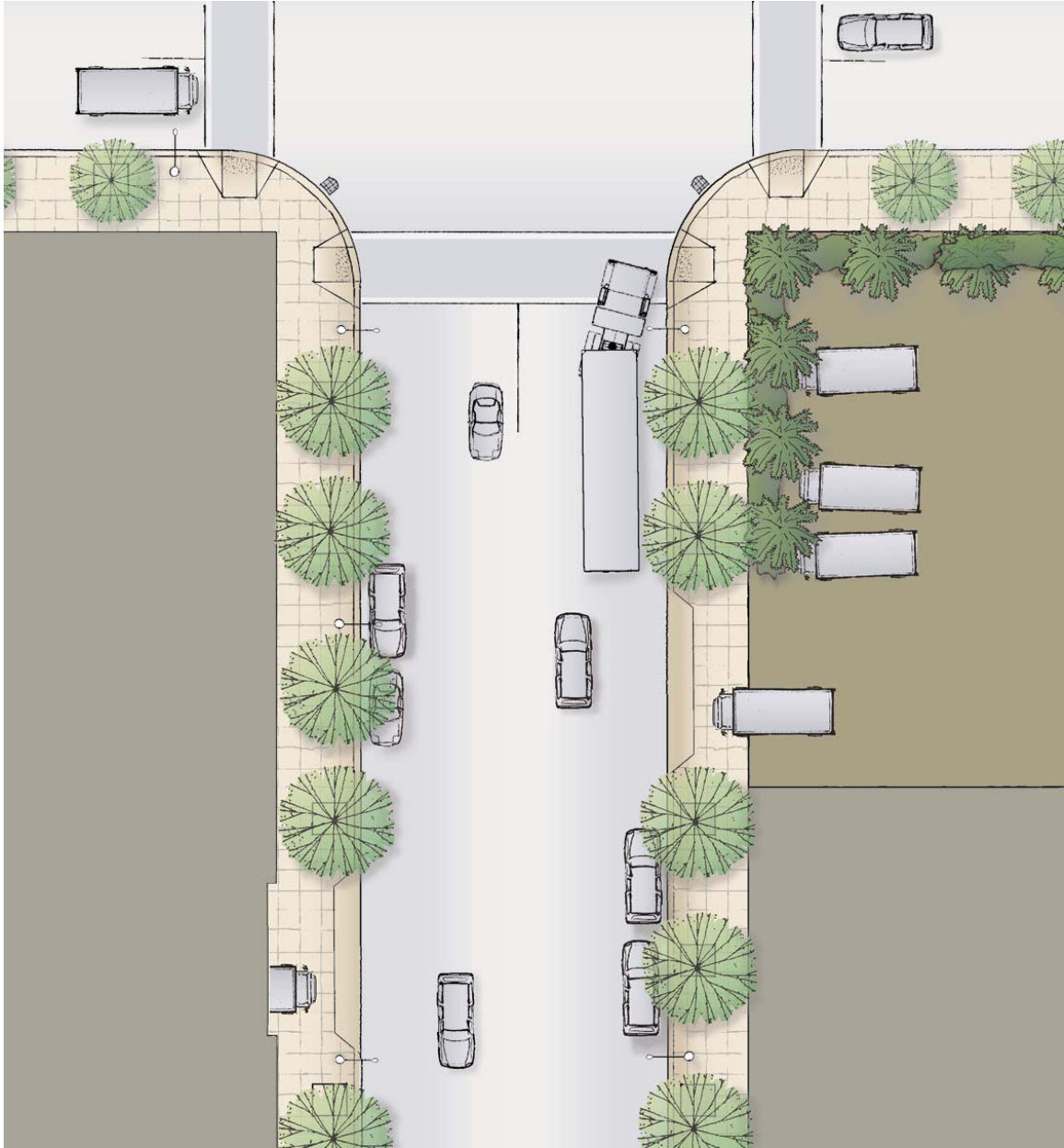
Figure E.4. Industrial street showing parking lot buffer plantings
